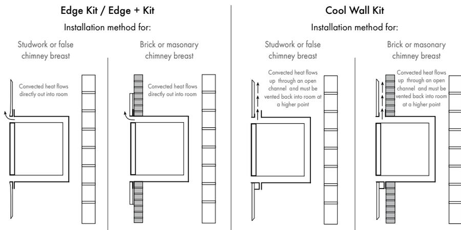
Please note: Diagram shows an Edge Kit. An Edge + Kit has an additional decorative frame that finishes the installation opening.
